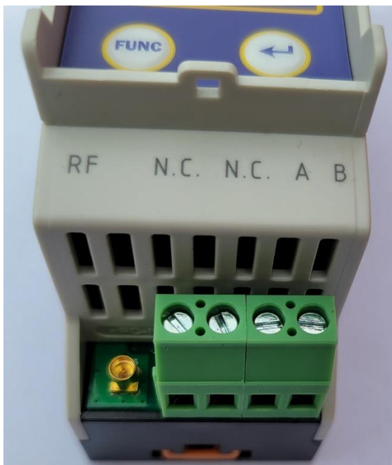
Bottom far Right B = Modbus RS485 Data B (-) Bottom Right A = Modbus RS485 Data A (+) RF = Antenna connection, push fit
